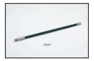
The 18 and 19 Series Precision Airlines are the most accurate impedance standards available today, and they are the recognized traceability path for impedance at high frequencies. Anritsu airlines are a critical component when measuring accurate impedances, enabling measurements down to 1.006 SWR to 18 GHz,1.01 SWR to 26.5 GHz, and 1.02 SWR to 40 GHz.
